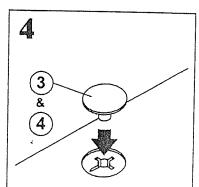
Attach Housing Caps (3,4) to all Klix Cam(2) by pushing neck of cap through center of cam.
